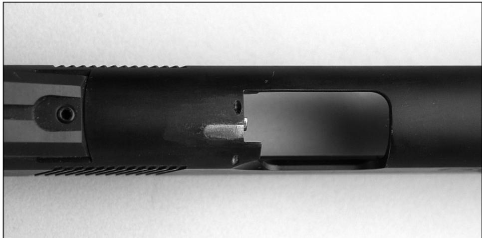
**The JPFO LC I unit can be positioned in two places. The first position is at the top of the slide. The second cants the installation of the unit 22 degrees to the right off the top dead center of the slide.**
